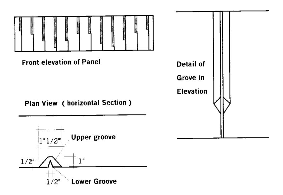
**9. Front of panel grooved**, top portion : 1 inch 1/2 wide, 45°, 1/4 inch flat bottom, lower portion with 45° funnel into narrower grove 1/2 inch wide to bottom of panel.
